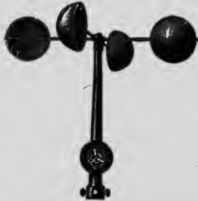
FIG. 131. — The anemometer. Inside the upright is a spindle to which the cross-bars are fastened. The wind pushes harder against the hollows of the cups than against the outsides, and thus turns the spindle. The stronger the wind, the faster the spindle whirls. A counting machine below is worked by the spindle and makes a record.
